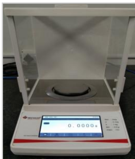
Analytical Balance with Density Kit Make-Wenser (MAB220T) Capacity-220g
