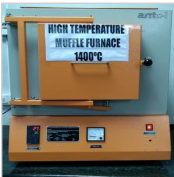
Make- ANTS LAB EQUIPMENTS Maximum Temperature-1400°C Heating rate- up to 15°C/Min
