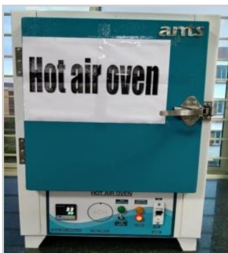
Hot Air Oven Make- ANTS LAB EQUIPMENTS Temperature range: RT to 300°C
